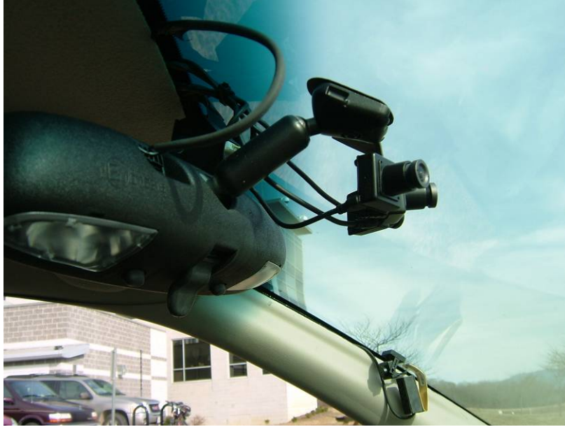
Figure 8. Forward Facing Cameras Mounted Behind the Center Rear View Mirror.
