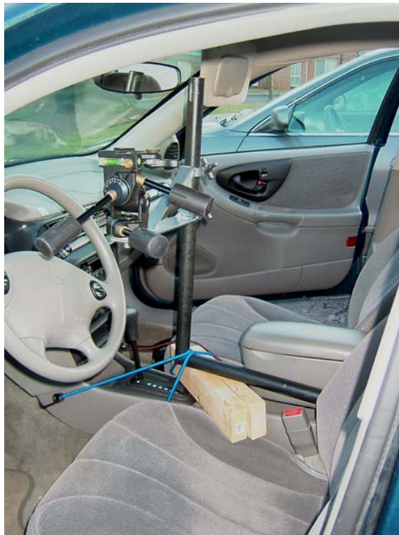
Figure 34. Bracket for Radiant Imaging CCD Photometer.
