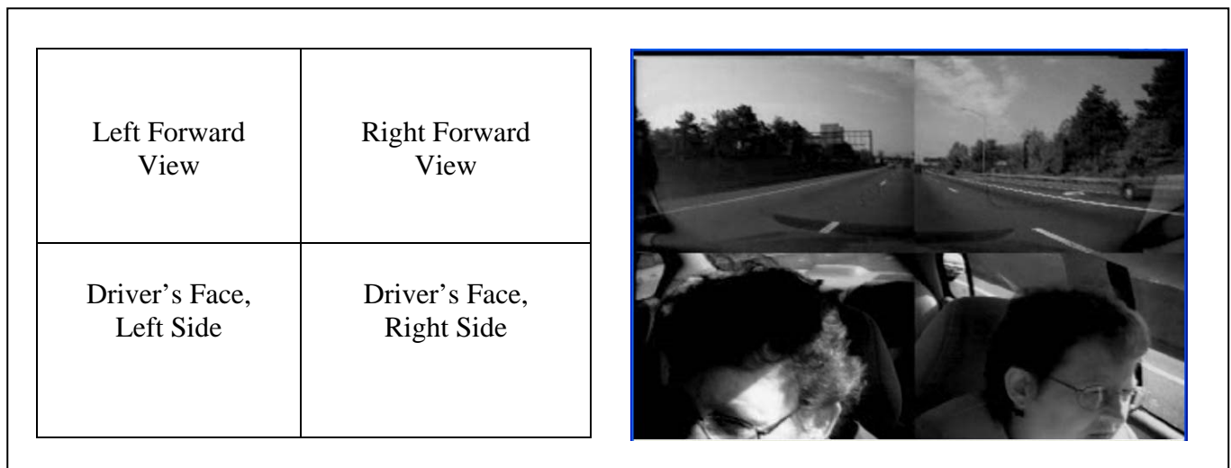
Figure 11. Diagram of Simultaneous Presentation of Four Camera Views.
