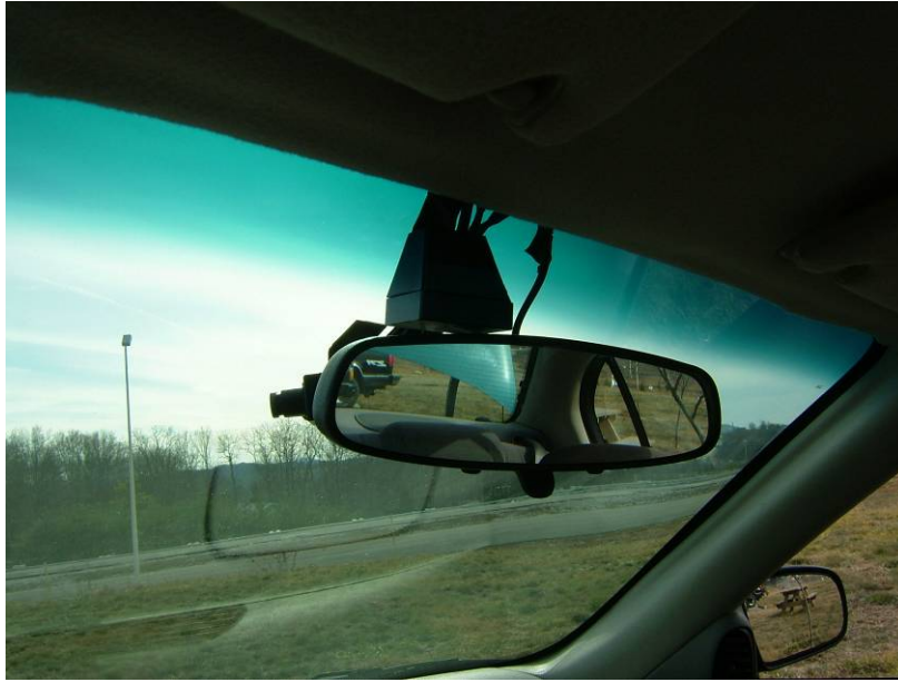
Figure 10. Driver Face Camera Mounted Above Rear View Mirror.
