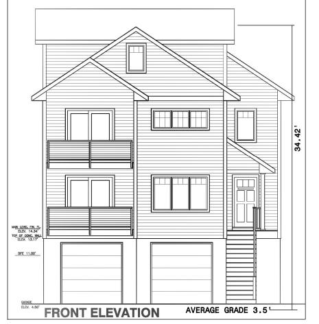
GARAGE FLOOR ELEVATION = 4.50TOP OF FOUNDATION WALL = 13.17BASE FLOOD ELEVATION = 11.00' MAIN FLOOR ELEVATION = 14.34
